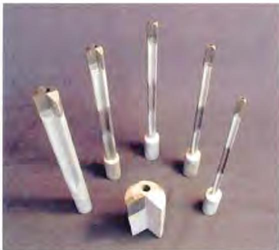
Carbide-tipped drills with a carbide insert drill head
