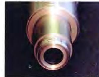
0.5" diameter hole through a 140" shaft
