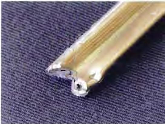
Damaged drill tip ready for re-tipping
